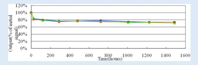
**High Temperature / High Humidity:** The following graph illustrates the signal output stability for a sensor exposed to  $+60^{\circ}$ C and 90% RH over 350 hours. The H<sub>2</sub>S concentration used was 10ppm H<sub>2</sub>S in air.
