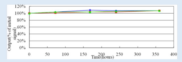
**Low Temperature:** The following graph illustrates the signal output stability for a sensor exposed to -20°C over 1500 hours. The  $H_2S$  concentration used was 10ppm  $H_2S$  in air.
