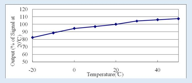
The following graph illustrates the typical effect of temperature on the zero offset of the NE4-H2S-200, with 2 standard deviation confidence limits
