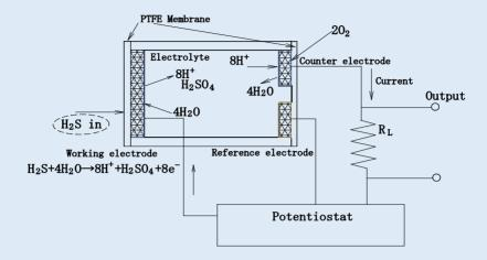
The NE4-H2S-200 consists of 3 porous noble metal electrodes separated by an acidic aqueous electrolyte, housed within a plastic (PPO) enclosure. Gas enters the cell via a gas phase diffusion barrier (capillary). An electrolyte reservoir ensures an excess of electrolyte is available at all times, and the sensor is vented to ensure that the internal and external pressure of the sensor is always in equilibrium.
