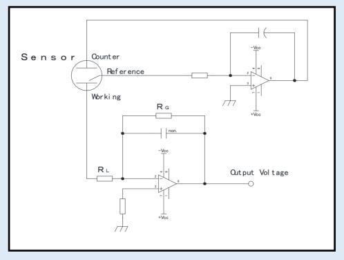
The basic measuring circuit for all 3-electrode electrochemical gas sensors is shown below:
