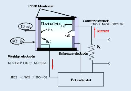
The NE7-NO2 consists of 3 porous noble metal electrodes separated by an acidic aqueous electrolyte, housed within a plastic (PPO) enclosure. An electrolyte reservoir ensures an excess of electrolyte is available at all times, and the sensor is vented to ensure that the internal and external pressure of the sensor is always in equilibrium.
