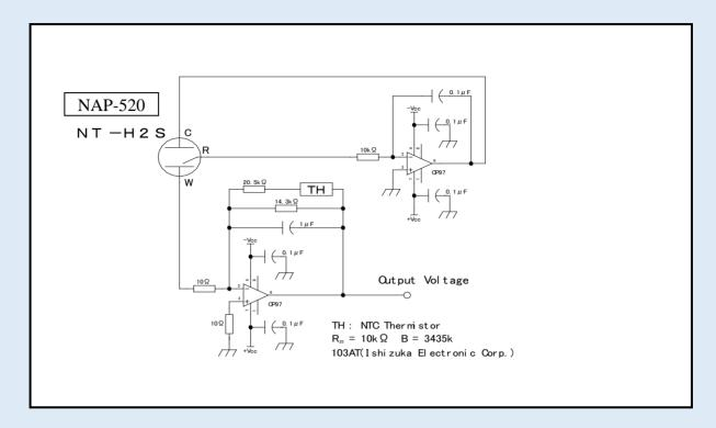
The circuit Nemoto employs for all its internal testing of NAP-520 is shown below:
