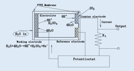
The NAP-520 consists of 3 porous noble metal electrodes separated by an acidic aqueous electrolyte, housed within a plastic (PPO) enclosure. Gas enters the cell via a gas phase diffusion barrier (capillary). An electrolyte reservoir ensures an excess of electrolyte is available at all times, and the sensor is vented to ensure that the internal and external pressure of the sensor is always in equilibrium.
