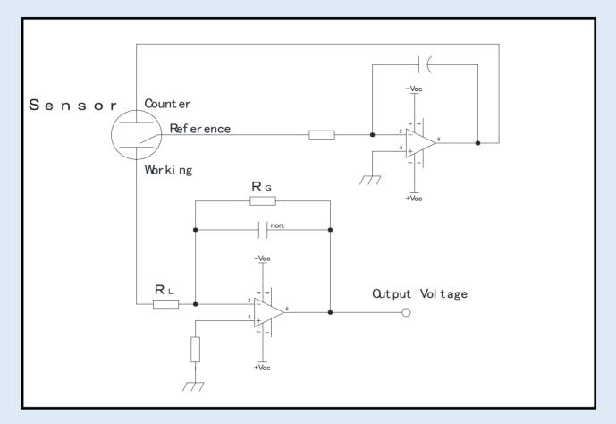
The basic measuring circuit for all 3-electrode electrochemical gas sensors is shown below:
