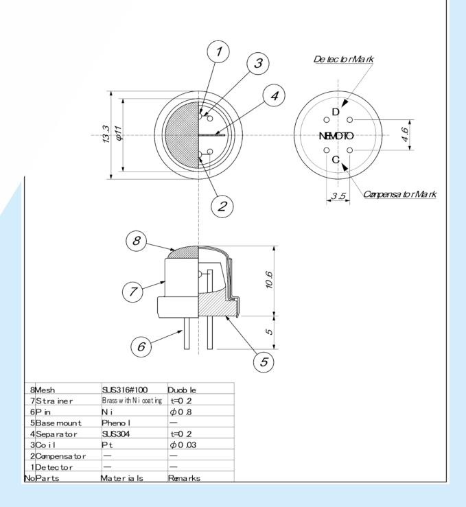
Test data on drift, poisoning, temperature performance, linearity are available on the Characterisation Document.
