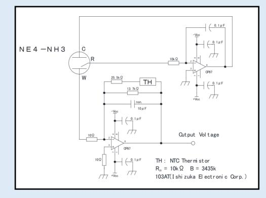
The circuit Nemoto employs for all its internal testing of NE4-NH3 is shown below:
