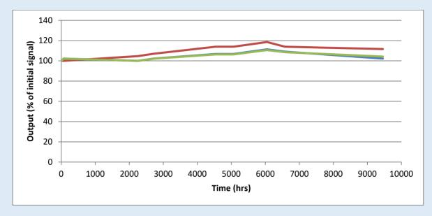
**High Temperature / High Humidity:** The following graph illustrates the signal output stability for a sensor exposed to  $+50^{\circ}$ C and 90% RH over 1100 hours. The NH<sub>3</sub> concentration used was 100ppm NH<sub>3</sub> in air.
