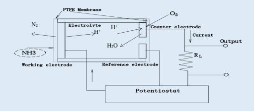
The NE4-NH3 consists of 3 porous noble metal electrodes separated by an acidic aqueous electrolyte, housed within a plastic (PPO) enclosure. Gas enters the cell via a gas phase diffusion barrier. An electrolyte reservoir ensures an excess of electrolyte is available at all times, and the sensor is vented to ensure that the internal and external pressure of the sensor is always in equilibrium.
