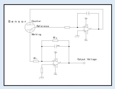
The basic measuring circuit for all 3-electrode electrochemical gas sensors is shown below:
