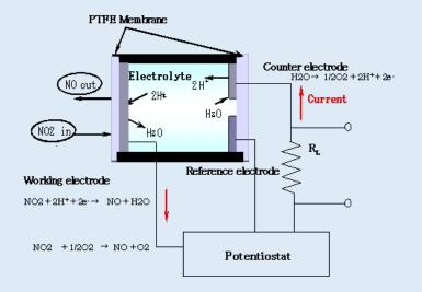
The NE4-NO2 consists of 3 porous noble metal electrodes separated by an acidic aqueous electrolyte, housed within a plastic (PPO) enclosure. An electrolyte reservoir ensures an excess of electrolyte is available at all times, and the sensor is vented to ensure that the internal and external pressure of the sensor is always in equilibrium.
