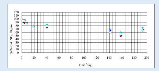
The following graph illustrates the signal output stability for a sensor exposed to  $-20^{\circ}$ C over 200 days. The NO<sub>2</sub> concentration used was 10ppm NO<sub>2</sub> in air.
