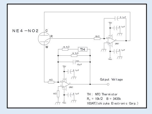
The circuit Nemoto employs for all its internal testing of NE4-NO2 is shown below:
