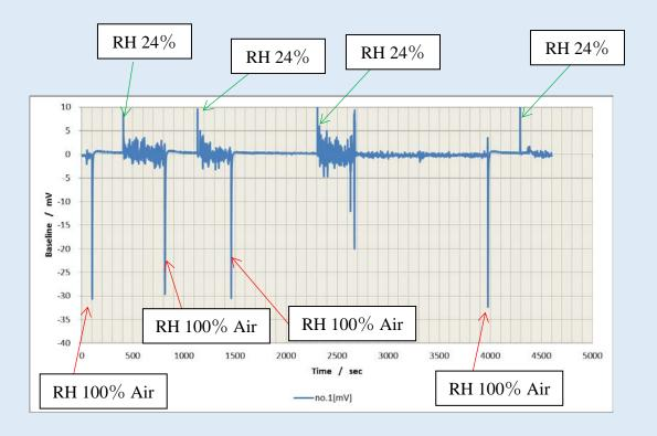
The transient spike response from the sensor for each humidity excursion was of approximately 5s in duration. The results here are expressed in mV from our recommended circuit, with 6mV being equivalent to 1 ppm NO<sub>2</sub>. The maximum amplitude of the spike when the humidity changed from low to high was 5 ppm equivalent, and -1ppm equivalent when humidity was changed from high to low.
