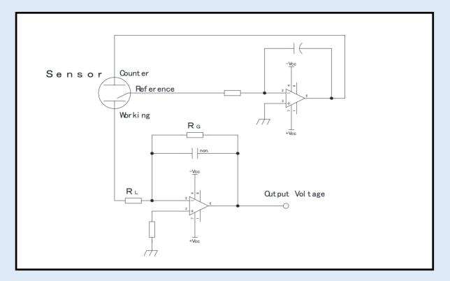
• In this arrangement, the output voltage =
