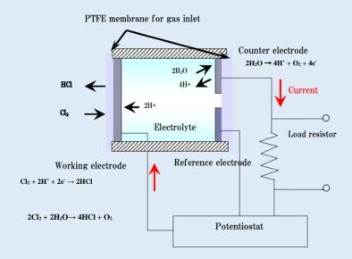
The NE4-CL2 consists of 3 porous noble metal electrodes separated by an acidic aqueous electrolyte, housed within a plastic (PPO) enclosure. An electrolyte reservoir ensures an excess of electrolyte is available at all times, and the sensor is vented to ensure that the internal and external pressure of the sensor is always in equilibrium.
