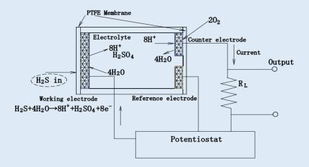
The NE4-H2S-500 consists of 3 porous noble metal electrodes separated by an acidic aqueous electrolyte, housed within a plastic (PPO) enclosure. Gas enters the cell via a gas phase diffusion barrier (capillary). An electrolyte reservoir ensures an excess of electrolyte is available at all times, and the sensor is vented to ensure that the internal and external pressure of the sensor is always in equilibrium.
