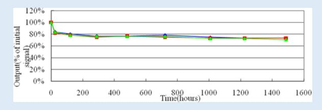
**High Temperature / High Humidity:** The following graph illustrates the signal output stability for a sensor exposed to  $+60^{\circ}$ C and 90% RH over 350 hours. The H<sub>2</sub>S concentration used was 10ppm H<sub>2</sub>S in air.
