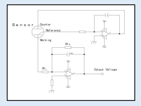
• In this arrangement, the output voltage =
