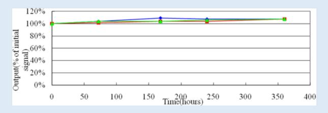
**Low Temperature:** The following graph illustrates the signal output stability for a sensor exposed to -20°C over 1500 hours. The  $H_2S$  concentration used was 10ppm  $H_2S$  in air.
