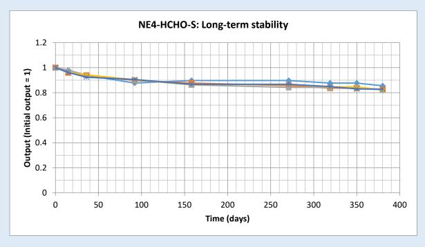
Measured in clean air at 20 deg C and 60% RH
