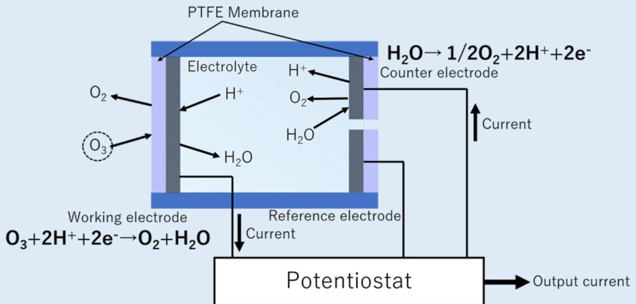
The NE4-O3 consists of 3 porous catalytic electrodes separated by an acidic aqueous electrolyte, housed within a plastic (m-PPE) enclosure. An electrolyte reservoir ensures an excess of electrolyte is available at all times, and the sensor is vented to ensure that the internal and external pressure of the sensor is always in equilibrium.
