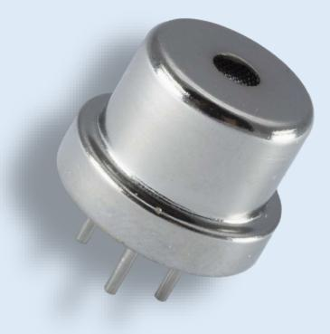
The NCP-180S-6S is a new Catalytic (pellistor) type flammable gas sensor supplied as a matched pair of pellistor elements mounted on a single header and protected by a metal enclosure and can.
