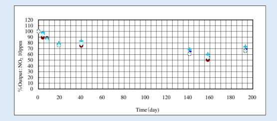
The following graph illustrates the signal output stability for a sensor exposed to -20°C over 200 days. The NO<sub>2</sub> concentration used was 10ppm NO<sub>2</sub> in air.
