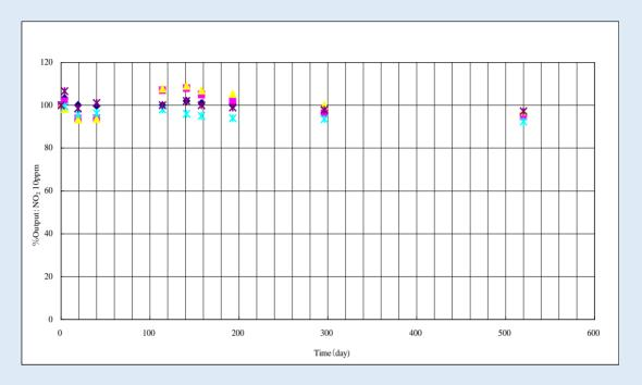
This data was generated in bench tests in a controlled clean environment. In service, in a real application, the long-term stability will also be dependent on the environmental conditions of the application.
