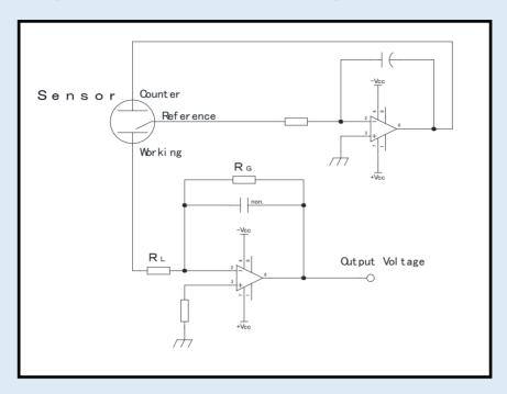
In this arrangement, the output voltage =
