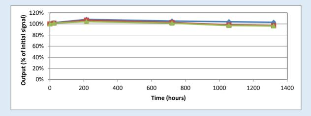
**Low Temperature:** The following graph illustrates the signal output stability for a sensor exposed to -20°C over 8000 hours. The H<sub>2</sub>S concentration used was 10ppm H<sub>2</sub>S in air.
