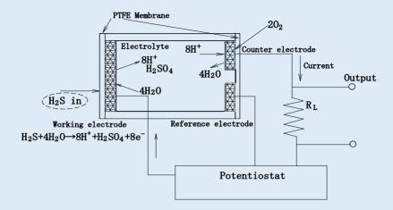
The NE4-H2S-100 consists of 3 porous noble metal electrodes separated by an acidic aqueous electrolyte, housed within a plastic (PPO) enclosure. Gas enters the cell via a gas phase diffusion barrier (capillary). An electrolyte reservoir ensures an excess of electrolyte is available at all times, and the sensor is vented to ensure that the internal and external pressure of the sensor is always in equilibrium.
