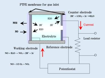
The NE4-NO consists of 3 porous noble metal electrodes separated by an acidic aqueous electrolyte, housed within a plastic (PPO) enclosure. Gas enters the cell via a gas phase diffusion barrier (capillary). An electrolyte reservoir ensures an excess of electrolyte is available at all times, and the sensor is vented to ensure that the internal and external pressure of the sensor is always in equilibrium.
