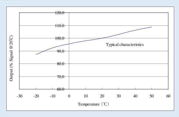
The following graph illustrates the typical drift of zero offset with temperature:
