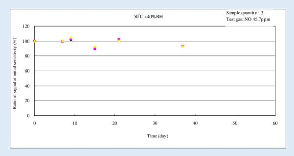
**High Temperature / Normal Humidity:** The following graph illustrates the typical signal output stability for a sensor exposed to +50°C and 60% RH over 50 days. The NO concentration used was 45.7ppm NO in air.
