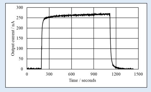
The following graph illustrates the typical response and recovery times for exposures to 0.5 ppm Ozone:
