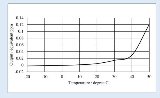
The following graph illustrates the typical effect of temperature on the zero output signal of the NE4-O3:
