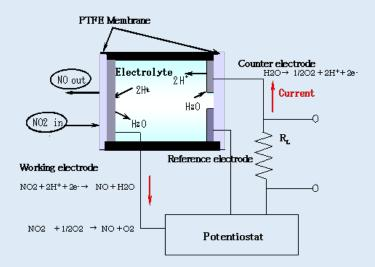
The NAP-550 consists of 3 porous noble metal electrodes separated by an acidic aqueous electrolyte, housed within a plastic (PPO) enclosure. An electrolyte reservoir ensures an excess of electrolyte is available at all times, and the sensor is vented to ensure that the internal and external pressure of the sensor is always in equilibrium.
